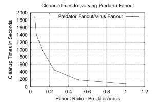
Figure 11. Clean up time as function of predator-to-virus fanout.
