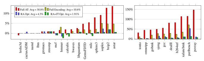
Fig. 3: Runtime overhead for SPEC 2006 compiled into position-independent executable (PIE) with different SAFER optimizations enabled. To improve readability, these results have been grouped into two charts, the left one with lower overhead benchmarks and the right including the rest.
