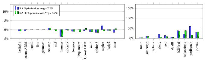
Fig. 4: Runtime overhead for non-PIE binaries. Only the two highest levels of SAFER optimization are shown.
