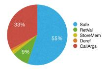
**Fig. 5:** The "Safe" area shows the percentage of jump tables that are transformed safely by SAFER in SPEC 2006 binaries (optimization O2). The rest are classified as unsafe, with the labels corresponding to the reasons listed in Sec. 5.2.
